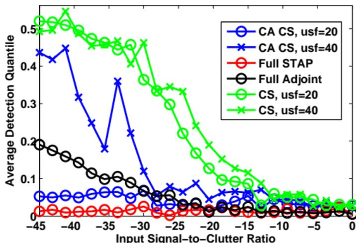
These results show that again, the fully-sampled STAP estimate performs better than all other techniques. Also, the  $20\times$  under-sampled CA CS estimate is shown to consistently achieve performance near that of the fully-sampled STAP and better than the fully-sampled adjoint.
