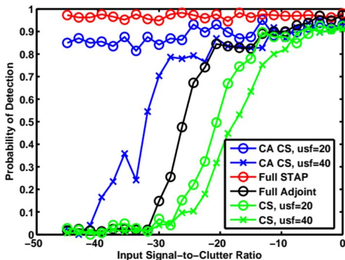
The CA CS method improves the probability of detection over the CS case and the fully-sampled matched filter case that does not use the covariance information. These results are shown with a probability of false alarm of .01.
