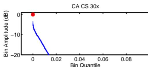
A comparison of solution methods applied to a problem with input SNR of 0 dB, input SCR of -20 dB. These plots show the relative amplitude of all the bins in the estimate produced by the identified technique.
