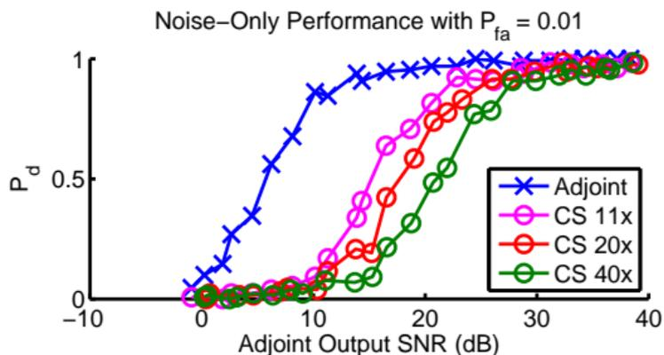
Compressed sensing detection performance degrades with subsampling rate. Each additional octave of under-sampling results in a raising of the noise floor by a factor of two, or 3 dB.
